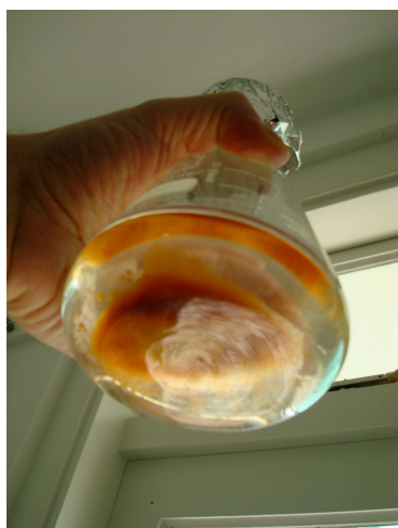
5: Residue settles at the bottom of the flask after separation. It can be removed by pouring the solution into a fresh flask or jar for refrigeration.
