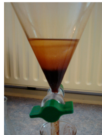
4: After a few hours syphon off the dark brown residue.
