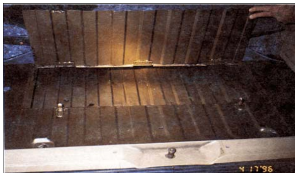
Welded compartment discovered in the rear of a minivan
