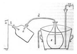
(a) is the worm tub, (b) the exit end of the worm, (c) the tubulated receiver, &c. Together with the gas, some solution of ammonia will escape and be collected in (c). The greatest attention must be paid to the fire which should on no account be withdrawn, otherwise the liquid in globe (e) will quickly be absorbed into the flask (c). When the gas passes over more slowly, the fire is somewhat noreased, and on no more bubbles appearing, the leaden tube is withdrawn from the globe and placed
